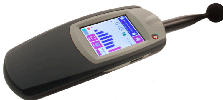
Figure 2. The Bedrock SM50 STIPA meter [7]. Whereas this instrument was originally developed as a STIPA meter, and has basic as well as more advanced STIPA features, it also includes other acoustic measurement modules, such as a real-time spectrum analyzer, RT60 meter and a sound pressure level meter.
