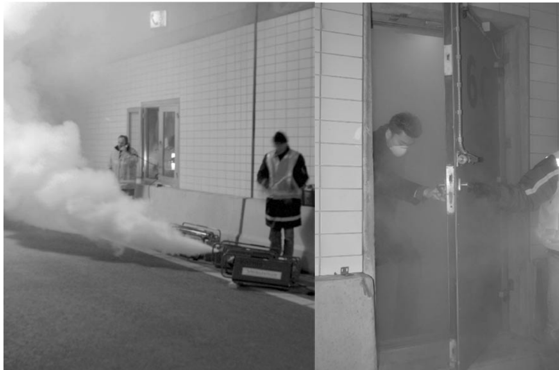
Figure 6. Smoke generation (left) and a test participant leaving the smoke-filled tunnel.
