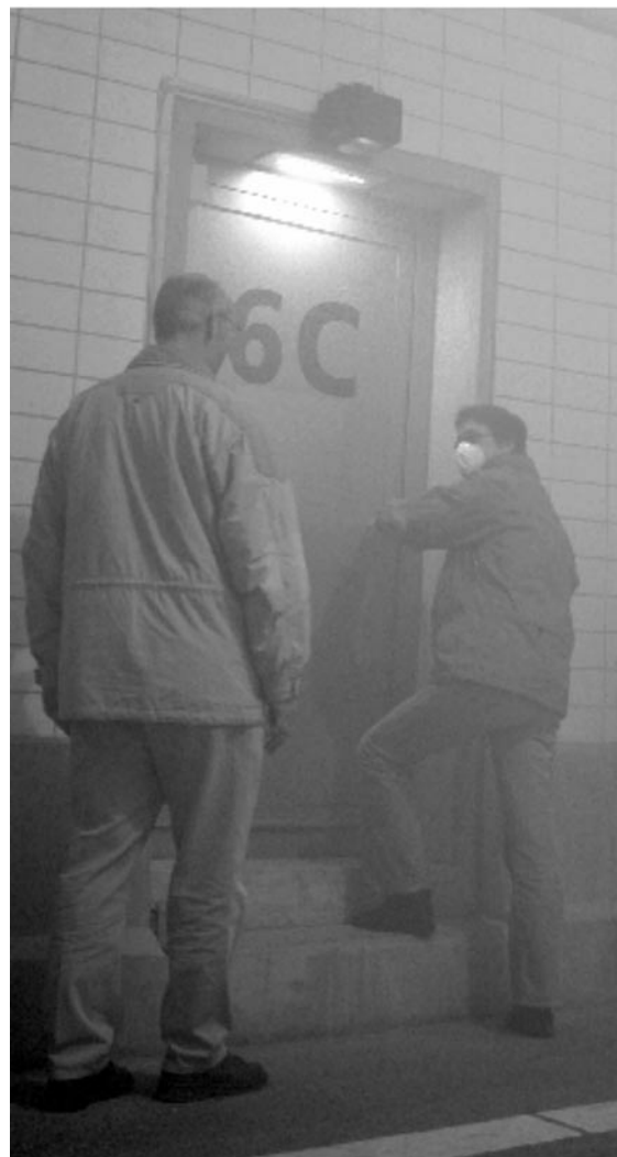
Figure 3. Emergency exit with sound beacon on top (black box; test assistants are preparing the area; smoke is starting to develop).
